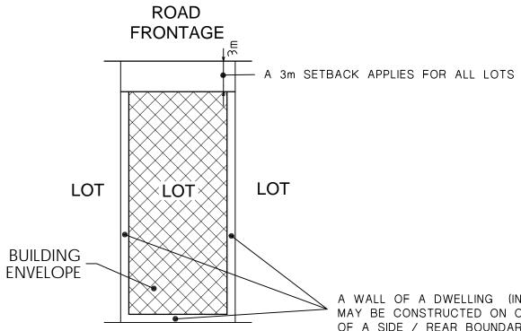
A WALL OF A DWELLING (INCLUDING GARAGE) MAY BE CONSTRUCTED ON OR WITHIN 200mm OF A SIDE / REAR BOUNDARY, OTHERWISE A MINIMUM 1 METRE SIDE SETBACK WILL APPLY.
