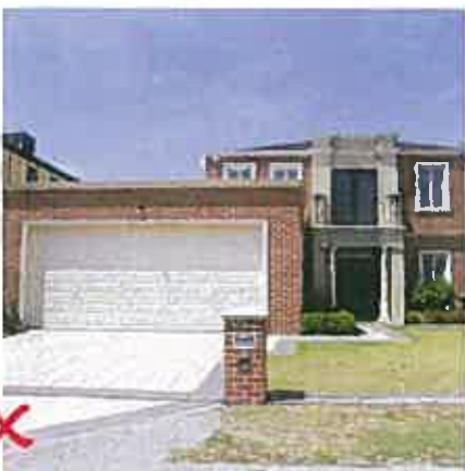
Example of non-compliant treatment for garage, set far from the main built form.
