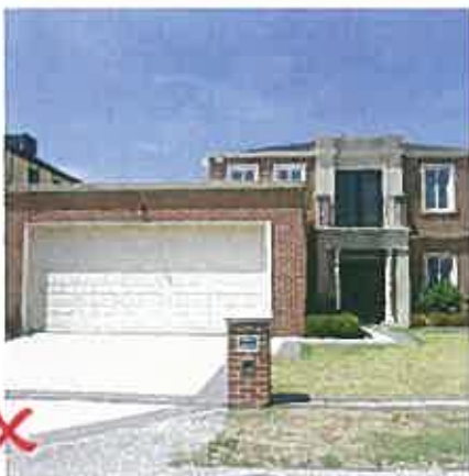
✗ Example of non-compliant treatment for garage, set forward from the main facade.
