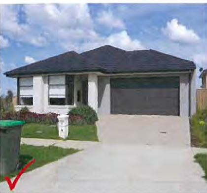
Garage setback from street frontages and behind front wall of the home
