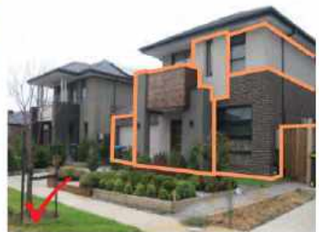
Articulated building forms
