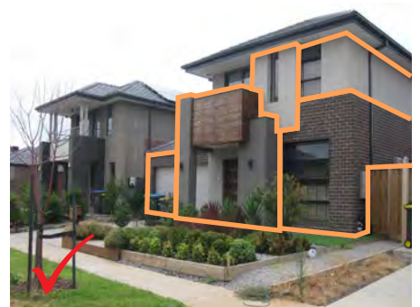
Articulated building forms
