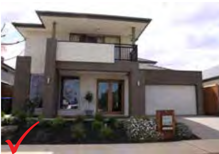
Double storey swelling with garage incorporating 1.5m covered verandah/ balcony, hence not requiring setback between the front wall and garage.
