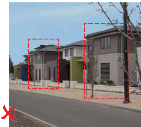
Example of non compliance facades, identical facades too close together
