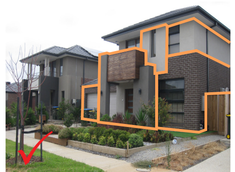
Articulated building forms
