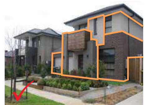
Articulated building forms
